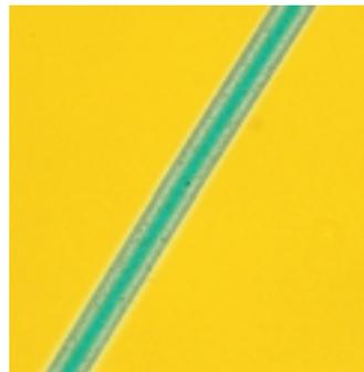
The unstained polymer fiber is only indistinctly visible in brightfield (left) but can be seen in detail in polarized light (center). The lambda plate (right) converts contrast to colors.
